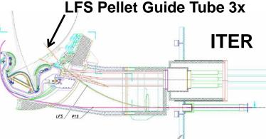
New ITER like LFS injection line installed and tested on DIII-D. 1.3mm pellets injected appear to trigger ELMs.
