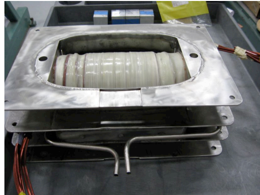
Racetrack bobbin welded to wound solenoid
