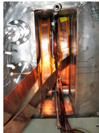
Test fit with all coils
