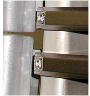
Re-designed current straps showed no melting after long-pulse operation
