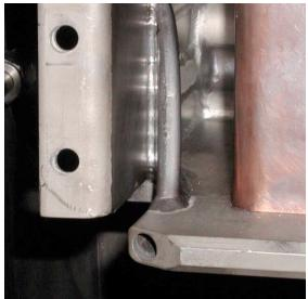
Localized melting observed after several 0.5 - 0.8 MJ pulses during 2003 operation
