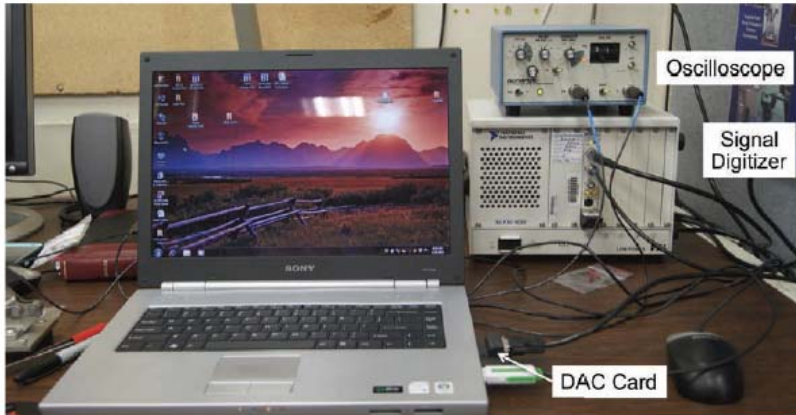
Figure 1. Photograph of the analysis computer, pulser, and digitizer.
